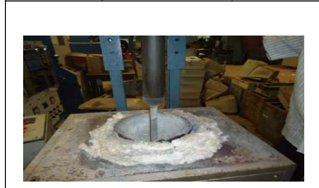
Figure: 3. Electrical Resistance Furnaces with a Stirring Assembly
