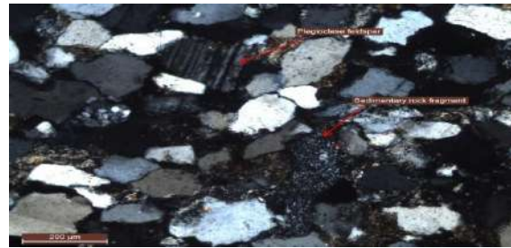
Figure 2: Photo of Petrographic Thin Section of the rock sample showing Plagioclase Feldspar and Sedimentary Rock Fragment.
