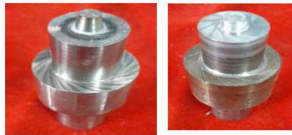
Figure: 2. Taper Cylindrical & Threaded tool pin profile
