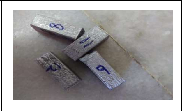
Figure: 4. Experimental Specimens – Impact test
